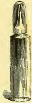
Small test bottle, with capillary orifice. § 139.
